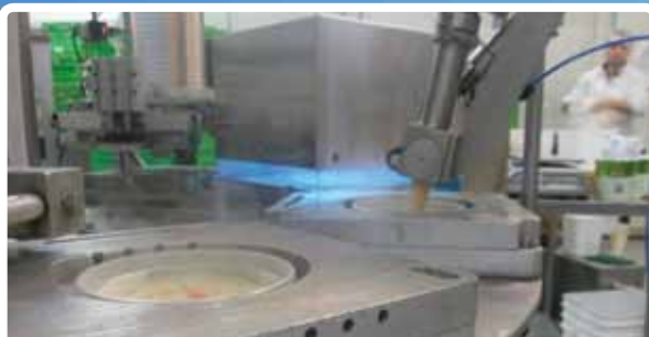
A retrofittable solution to surface disinfection of moulds, yeasts and bacteria installed with custom SS housing onto existing processing lines.
